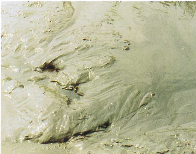
Close-up of slurry being pumped which comprises pulverized coal, fly ash, sand and clay.
