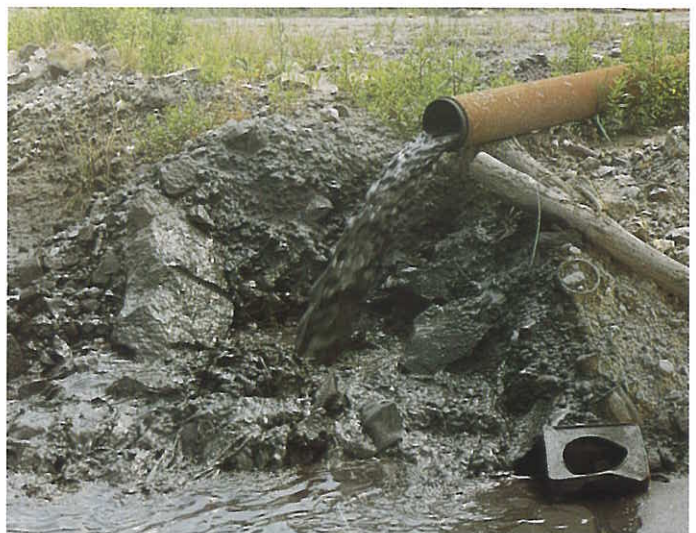
Discharge pipe showing type of slurry being pumped.
